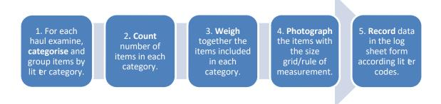
**Diagram 1.** Basic step sequence for recording seabed litter data on board. The concept of Item refers to each object (complete or in fragments) that constitutes a waste recovered from the seabed. The category mainly refers to the type of items, grouped according to the material they are made of, the use of the items or other aspects of their composition (Adapted from ICES, 2022).
